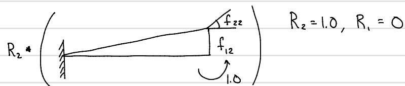
\* Stiffness superposition apply displacements
