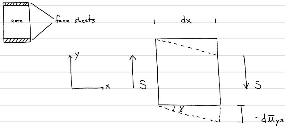
$$\text{Shear strain } \gamma = -\frac{d\bar{y}_s}{dx}$$
