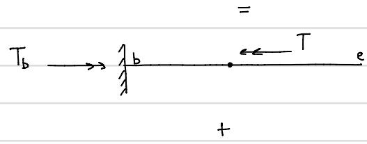
remove redundant, apply loading
