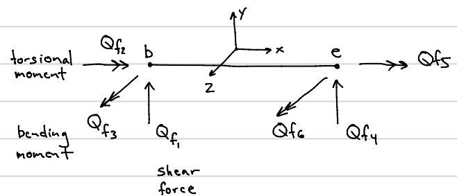
How to derive fixed-end forces for torsion?
