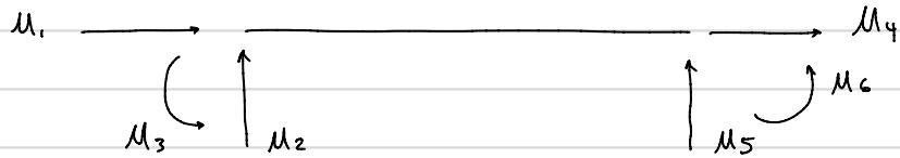
$$\{M_T\} = \begin{Bmatrix} 0 \\ 0 \\ -\Theta_T \\ \Delta_T \\ 0 \\ \Theta_T \end{Bmatrix} = \frac{\alpha L}{2} \begin{Bmatrix} 0 \\ 0 \\ -(T_b - T_+)/d \\ (T_b + T_+)/d \\ 0 \\ (T_b - T_+)/d \end{Bmatrix}$$
