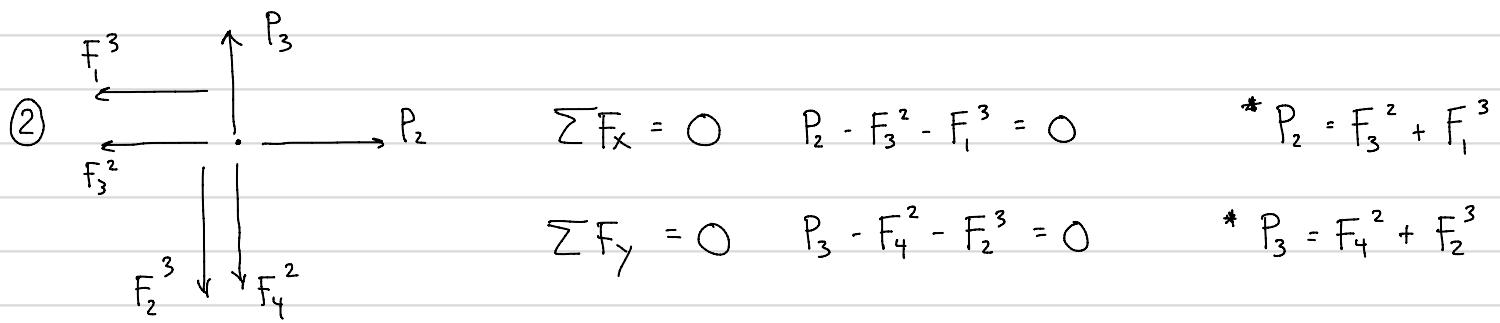
$$\begin{aligned} \sum F_x &= 0 & P_2 - F_3^2 - F_1^2 &= 0 & *P_2 = F_3^2 + F_1^2 \\ \sum F_y &= 0 & P_3 - F_4^2 - F_2^2 &= 0 & *P_3 = F_4^2 + F_2^2 \end{aligned}$$
