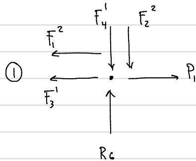
$$\begin{aligned} \sum F_x &= 0 & P_1 - F_3^1 - F_1^1 &= 0 & *P_1 = F_3^1 + F_1^1 \\ \sum F_y &= 0 & R_6 - F_4^1 - F_2^1 &= 0 & R_6 = F_4^1 + F_2^1 \end{aligned}$$
